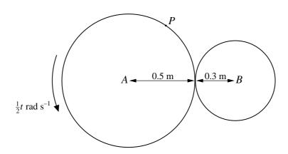
Two coplanar discs, of radii 0.5 m and 0.3 m, rotate about their centres A and B respectively, where AB = 0.8 m. At time t seconds the angular speed of the larger disc is  $\frac{1}{2}t \operatorname{rad} \operatorname{s}^{-1}$  (see diagram). There is no slipping at the point of contact. For the instant when t = 2, find
